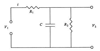
We set the numerical values of C and  $R_2$  equal to 1. Let us consider the voltage  $V_1$  as an input and the voltage  $V_2$  as an output. Taking  $V_2$  and the current i as the descriptor state variables  $\xi_1$  and  $\xi_2$ , respectively, we can represent the system by
