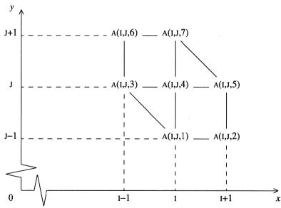
Important: the user must provide the matrix A only on the finest grid. The coarse-grid matrices are computed internally by the routine by means of Galerkin approximation.
